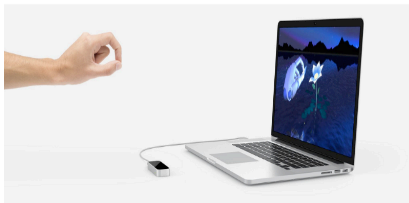
Fig 1: Leap motion usage. The small object in the middle is Leap Motion Controller connecting to the Mac on the right. Hand on top of the Leap Motion is tracked and interacted with virtual objects
