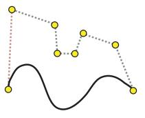
**Solution:** Consider the straight line shown in the figure below. This line intersects the control polygon and the Bézier curve in two (square) and four (circular) points. This violates the *variation diminishing property*, and, as a result, this Bézier curve is incorrect. Moreover, since a portion of the curve is not in the convex hull of the control points, this violates the convex hull property.
