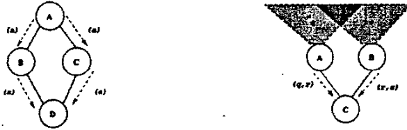
Figure 5. The implosion and overlap problems associated with classic flooding [10]
