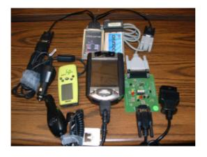
Figure 3: TrafficView prototype hardware components
