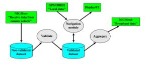
Figure 4: The structure of a node in TrafficView
