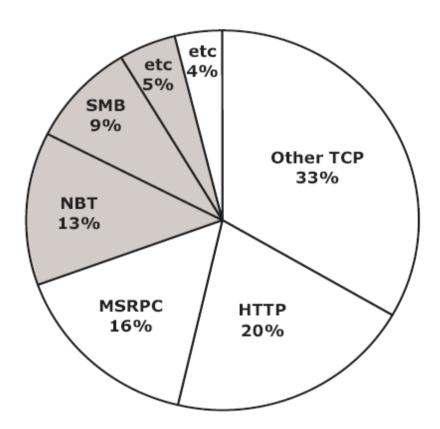
Figure 2: Traffic Volume Distribution on Sample User Machine (gray slices not captured)
