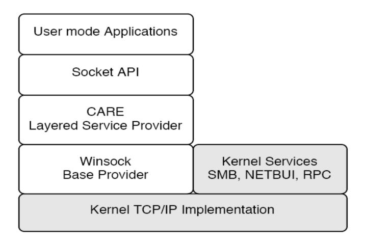
Figure 1: Layered Service Provider in Windows XP Stack
