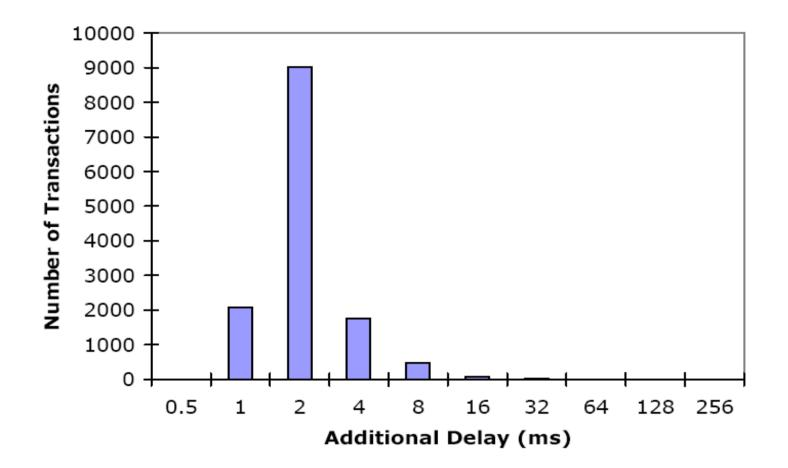
Figure 5: Replay Performance Between 2 Machines over Ethernet (rounding up to next delay bin)
