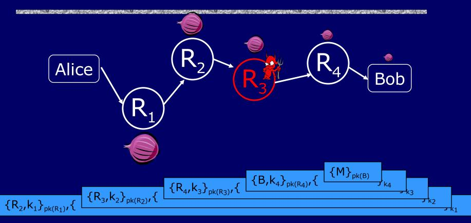
Routing info for each link encrypted with router's public key
